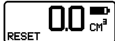
The meter is shut off by pressing the left button for 2 seconds.
