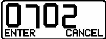
Press ENTER (left button) to accept and save the new calibration, or CANCEL (right button) to cancel the changes and return to the old calibration factor.
