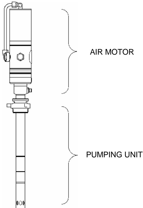
The piston diameter of the air motor is 75 mm (~ 3"). The motor consists of an air cylinder with piston and one reciprocal valve. The valve directs the compressed air alternately to the top or bottom of the piston, thus producing a reciprocating motion of the air motor piston rod.
