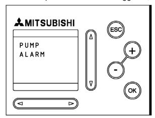
The system stops lubricating and the alarm contact closes.
