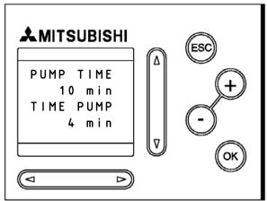
In this example 4 minuter has passed of the pump time.
