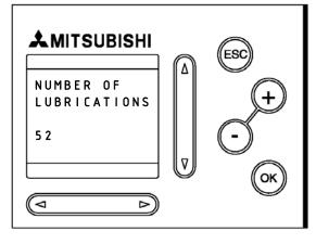
In this case 52 complete lubrication cycles of both lines have been performed.
