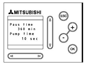
Increase the pause time by stepping it up with the + button until it equals the set pause time. Push the OK button to confirm.
