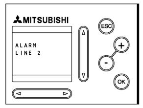
In this case the pressure switch confirmation has not been obtained during the pressurising of Line 2.
